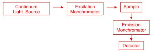
The intensity of fluorescence is strongly dependent on the number of excited state species. Since this excitation is the result of absorbance of a photon, a greater number of photons incident on the sample will lead to stronger fluorescence. Absorbance measurements are actually more difficult with very intense sources, as you will be comparing small differences between relatively large numbers.
