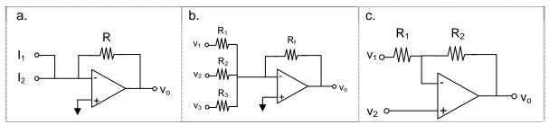
8. Given the circuit below, what output would you expect for a 1.25 mA input current? Derive the relationship between v<sub>o</sub> and i<sub>in</sub>. How would you redesign this circuit to make it suitable for measurement of low current signals (micro- to nano-amp signals)?
