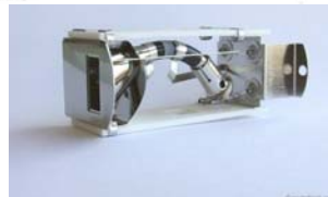
Figure 13-2 (a) Discrete dynode electron multiplier. Dynodes are kept at successively higher potentials via a multiplying voltage divider. (b) Continuous dynode electron multiplier. (Adapted from J. T. Mason, Introduction to Mass Spectrometry, p. 247, New York: Raven Press, 1985, 1998, permission.)
