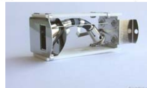
Figure 11-2 (a) Discrete dynode electron multiplier. Dynodes are kept at successively higher potentials via a multistage voltage divider. (b) Continuous dynode electron multiplier. (Adapted from J. T. Mason, Introduction to Mass Spectrometry, p. 247, New York: Raven Press, 1985, 1998 permission.)
